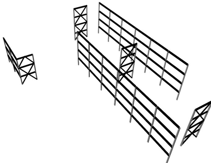
**Structural Depth – Final Lateral System Design Summary (continued)****Special Concentrically Braced Frames – C, E, G, K.6]**
