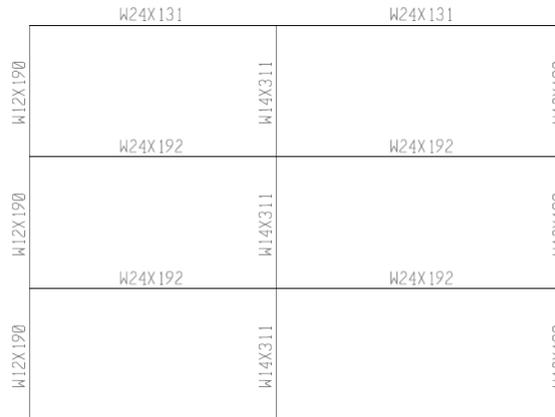
All of the beams in Special Moment Frame 8 have the same details for connections and bracing, the only difference is that they are different W-shape sections. The typical reduced beam section connection used in SMF-8 has the following values and the spacing of bracing is also given. The bracing assumes shear studs spaced at 12" between the protected zones. (See the appendix for more detailed information):
