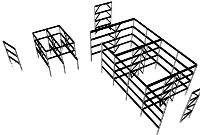
Redesigned Lateral System (Seismic) – Seattle, WA
